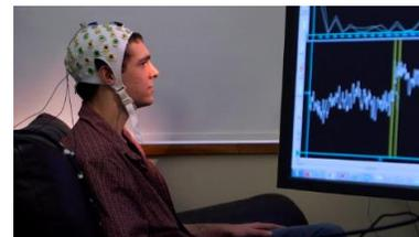
read signals from the brain and use computer chips and programs to translate the signals into action. [Researchers](#) in Germany designed a BCI-controlled wheelchair and tested it in 15 healthy subjects. Their results suggest BCIs are feasible for wheelchair control, however data also revealed a number of design issues that require further modifications and study.
